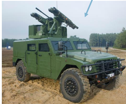
Firing management system on light ground vehicle
